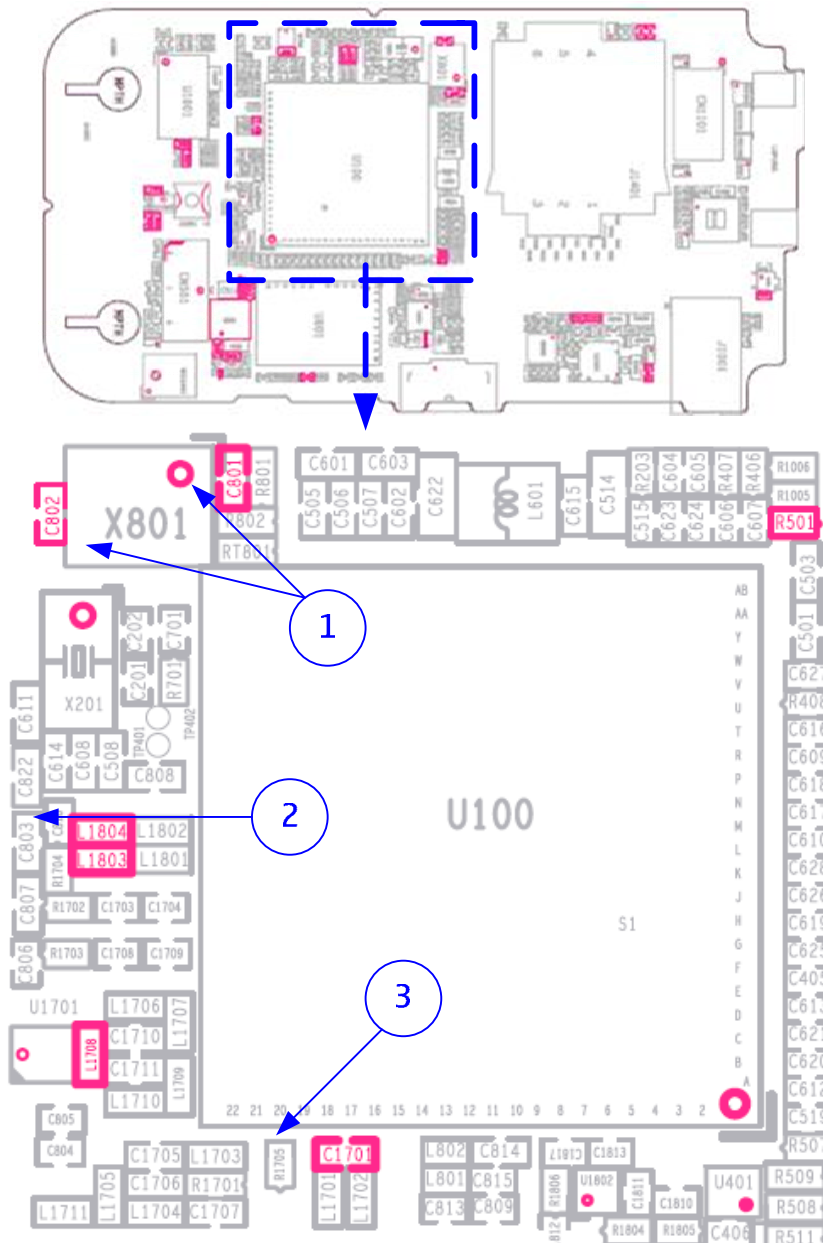
Figure 3 RF RX voltage checking test point
